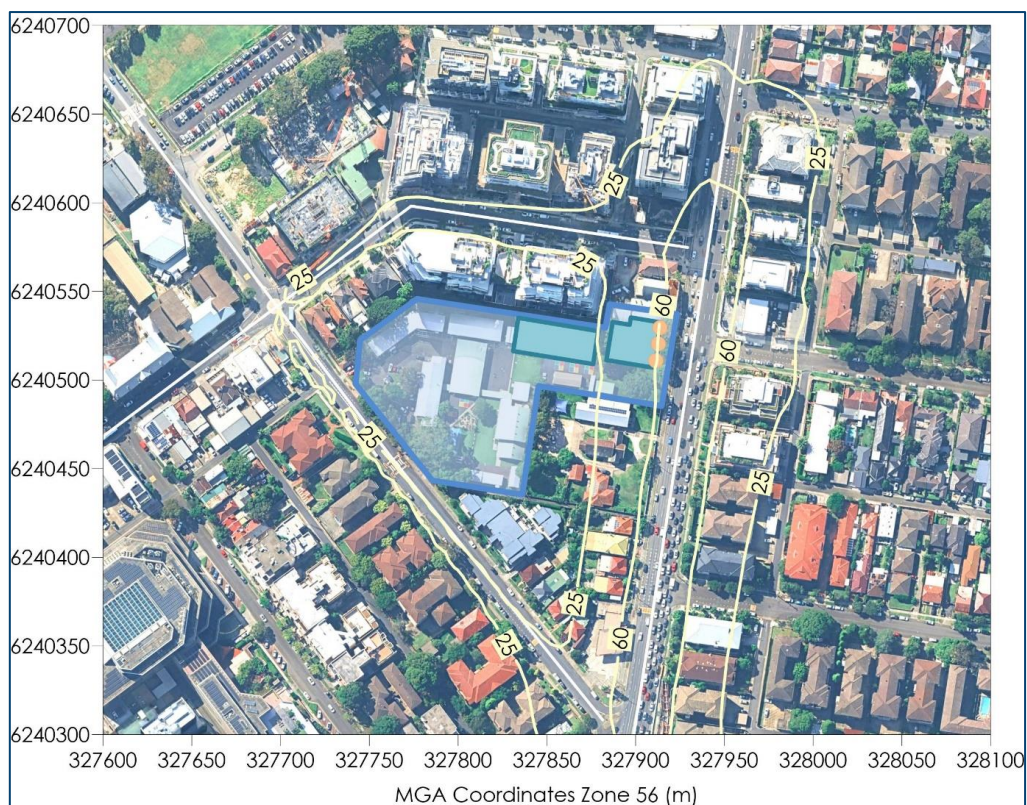
Figure 6-5: Predicted incremental 1-hour average NO 2 concentrations (µg/m³)
