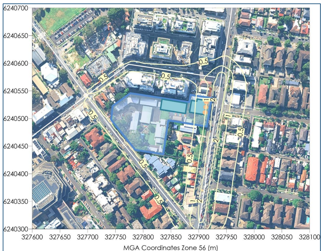
Figure 6-3: Predicted incremental 24-hour average PM_{2.5} concentrations ( \mu g/m^3 )
